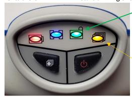
When the receiver gets a FLOAT solution (resolves integer ambiguities) the YELLOW LED will start to flash. When the receiver is fixed the YELLOW LED will continuously lite.
