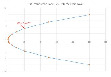
1 foot above your GNSS antenna, the beam width is 1.6' in diameter. 20 feet above the rover antenna (perhaps the midpoint of tree canopy), the 1st Fresnel beam diameter is 7 feet! A clearing in the treetops 100' above your antenna needs to be 16' in diameter.
