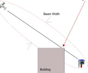
Clear path means that you don't just need a small opening in the trees for a laser beam to shoot through. You need an opening in the trees large enough that most of the energy which is spread out over the Fresnel beam width reaches the receiver with no obstructions.
