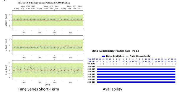
The position trends are very stable and are within 1 cm horizontal and vertical of the published IGS08 positions. The average locations and all of the error bars are fully contained in the green error bands. Coupled with continuous recent Data Availability this station appears be a great CORS resource.
