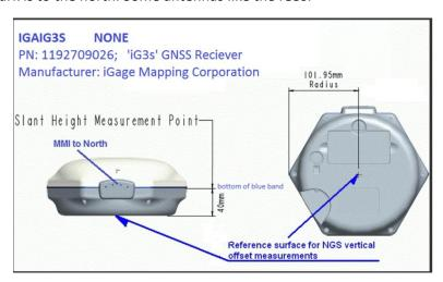
Have the MMI (Man-Machine-Interface) rotated to the north.
