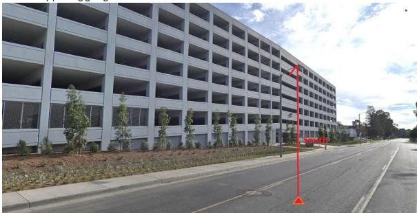
This is a **bad** location because the structure completely blocks the antenna's view to the South and East:
