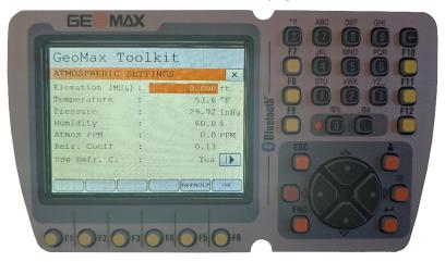
The purpose of this screen is to compute an Atmospheric PPM correction and enable/disable compensation for refraction.
