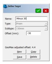
When a prism is entered in SurvCE, the standard Absolute offset is entered. SurvCE computes the GeoMax (Leica) adjusted offset as
