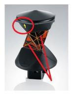
There is a 0.005 meter (5 mm, 0.016 foot) vertical offset between adjacent prism faces on the ZPR1 360 prism.
