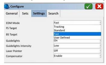
The default mode is 'Standard'. If you handhold the prism rod close (less than 50 feet from the robot) to the gun, the robot will lose sight of prism if you wobble the prism while the EDM is fired. (Because tracking is turned off in Standard mode when the EDM fires.)
