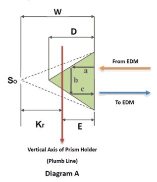
The distance that we want to measure is the distance from the instrument center (vertical axis) to the vertical axis (plumb line, Diagram A) of the prism holder.
