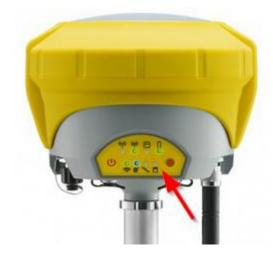
13. Now the rover is storing the kinematic raw data. To store a point just press the Measure button
