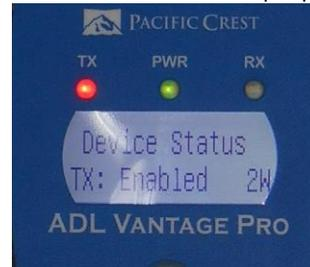
On hot days, it is possible that the radio power setting is higher than the enabled value. Power will also be reduced if Antenna Detect is enabled and a fault is detected.
