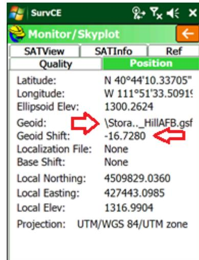
The Geoid Shift should be negative and the Local (orthometric) elevation should be above the Ellipsoid elevation as shown above.
