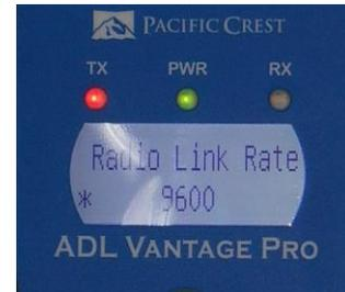
NOTE: 50% of all RTK Radio Problems are due to incorrect Radio Link and Serial Baud Rate settings. To reduce the chance of bad configurations we have forced all of the baud rates to be 9600. (In other words, the answer is always 9600 for the Internal CHC radio.)
