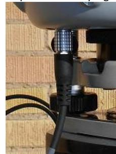
4. Connect the Y connector power cable to the battery. DOUBLE CHECK THE POLARITY (RED to +) (BLACK TO -) and then plug in the radio Y connector.
