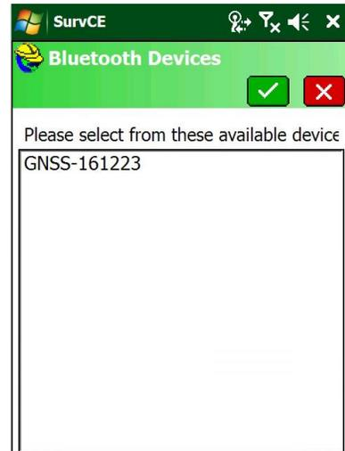
12. Highlight the correct receiver (the number is the serial number of the device, if you have your Base AND Rover powered up, make sure you are connecting to the Rover!)
