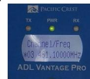
The rover frequency must match the frequency selected on the base. Noted that the rover
