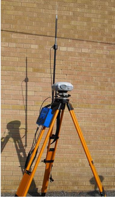
Set the UHF radio antenna to the North of the GPS receiver.
