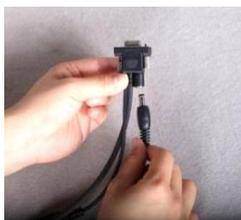
Connect the Power Adapter socket to the mains 100-240 VAC and Power Adapter male Jack connector to the Power Port of the GPS to PC cable.
