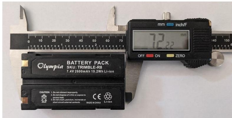
A battery is too long if you have to push the battery into the battery slot with high force in order to have the retaining clip secure the battery end.
