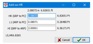
The top line "20.8072m 6.82651" shows the last processed HR in the file in meters and feet (the shot at the very bottom of the file.)
