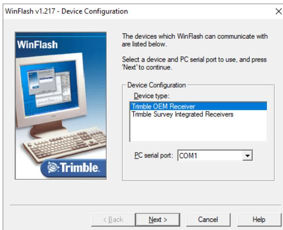
Choose the correct PC Serial Port. Select 'Trimble OEM Receiver' if there is more than one option.
