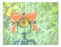
When the scope inverts for the reverse shot, there will be double lines on the right, instead of a single line. Carefully center the double lines over the black arrow.
