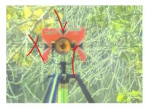
In this case I will use the top and right-hand black arrows to adjust the crosshairs to be EXACTLY (this is a 1" robot) at the center of the arrows.
