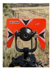
It is important to use a round prism with a target for the horizontal shot. It is best if the round prism is nearly 300 feet distant. Stepping off 100 paces is close enough.
