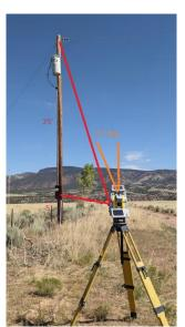
If the pole sticks out of the ground 30 feet, the telescope is 5 feet above the ground, then you will be set up between 12' (27 deg) and 49' (63 deg) from the base of the pole.
