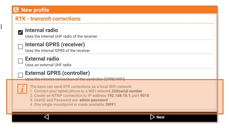
Instructions on how to connect the external application to the Zenith base are reported directly in X-PAD Ultimate software.
