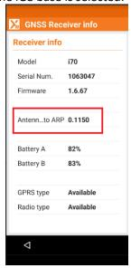
X-PAD is using 0.1150 meters which is 0.001 meters (0.003 feet) in error. This is close enough for GNSS work.
