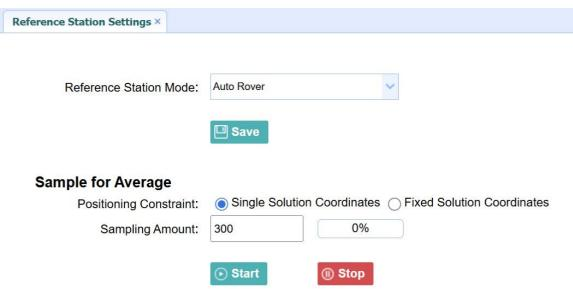
Use this screen to configure settings such as the station coordinates and the broadcast station identifiers. You must enter accurate information in these fields, as this data affects the accuracy of logged data files and broadcast correction data significantly:
