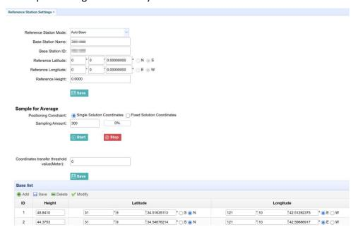
c) **Manual Base:** The receiver will serve as a base after this mode is enabled. Users need to configure the receiver manually.
