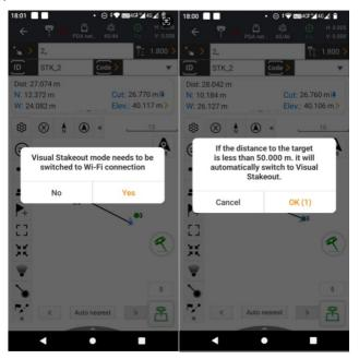
(3) In Vision Settings, we can adjust the switch distance: the front camera is used from 50 m to 3 m, and the bottom camera takes over within 3 m.
