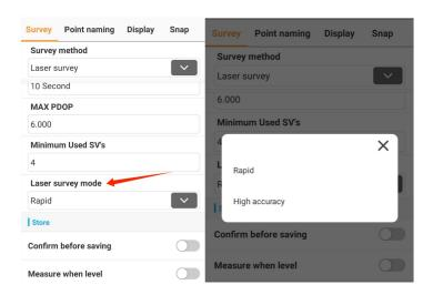
(6) Our software also supports automatic store. When the laser remains stationary for a certain period of time, the collection can be automatically completed. Users can customize the Max movement distance and time interval
