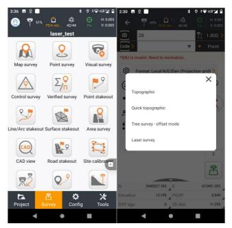
(2) After tapping Laser survey, you'll receive a safety-use notice and a laser initialization prompt. Follow the on-screen instructions to complete the laser initialization. To ensure survey accuracy, it is necessary to walk 6 meters or 3 meters and then return to the original position to complete the laser initialization.
