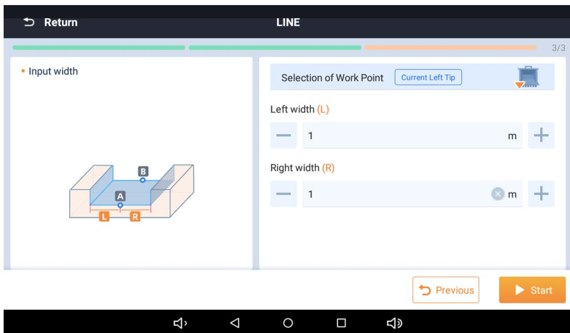
**Note: A width value of 0 creates an inclined plane design.**
